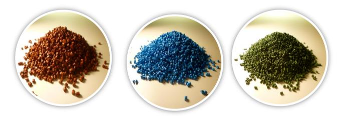
ColorFalt® is a pigment preparation that has been developed to solve the problems of working with powder pigment at an asphalt plant. The demand for a pelletized product came from the asphalt producers.
