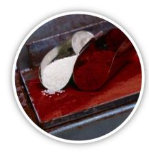
Red asphalt produced with ColorFalt® has a higher stability than standard mixtures. This can increase to a higher Marshall stability of 10%. The polymer also increases the softening point of the bitumen. The red asphalt mixes with ColorFalt® perform much better than asphalt without ColorFalt® over long periods of warm weather and for example on bridge decks and parking decks.
